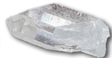
Quartz Crystals vibrate at a regular interval when exposed to an electrical current
