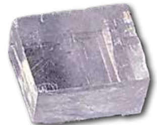
Optical Calcite splits light into two rays
